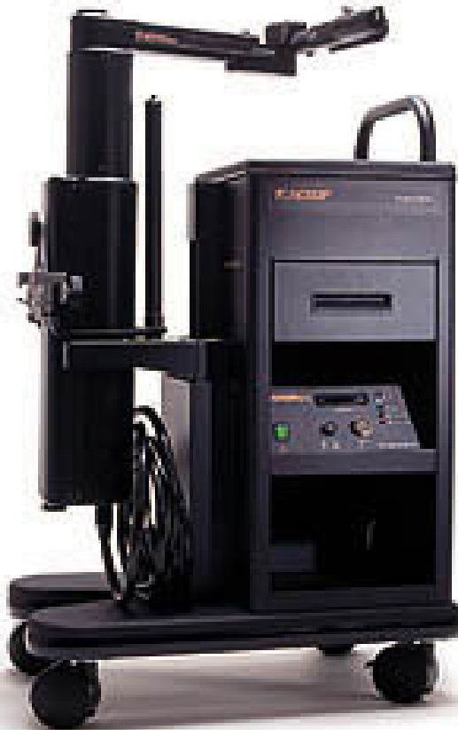
AESOP: Automated Endoscopic System for Optimal Positioning
