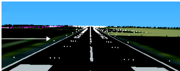
Runway edge lights
